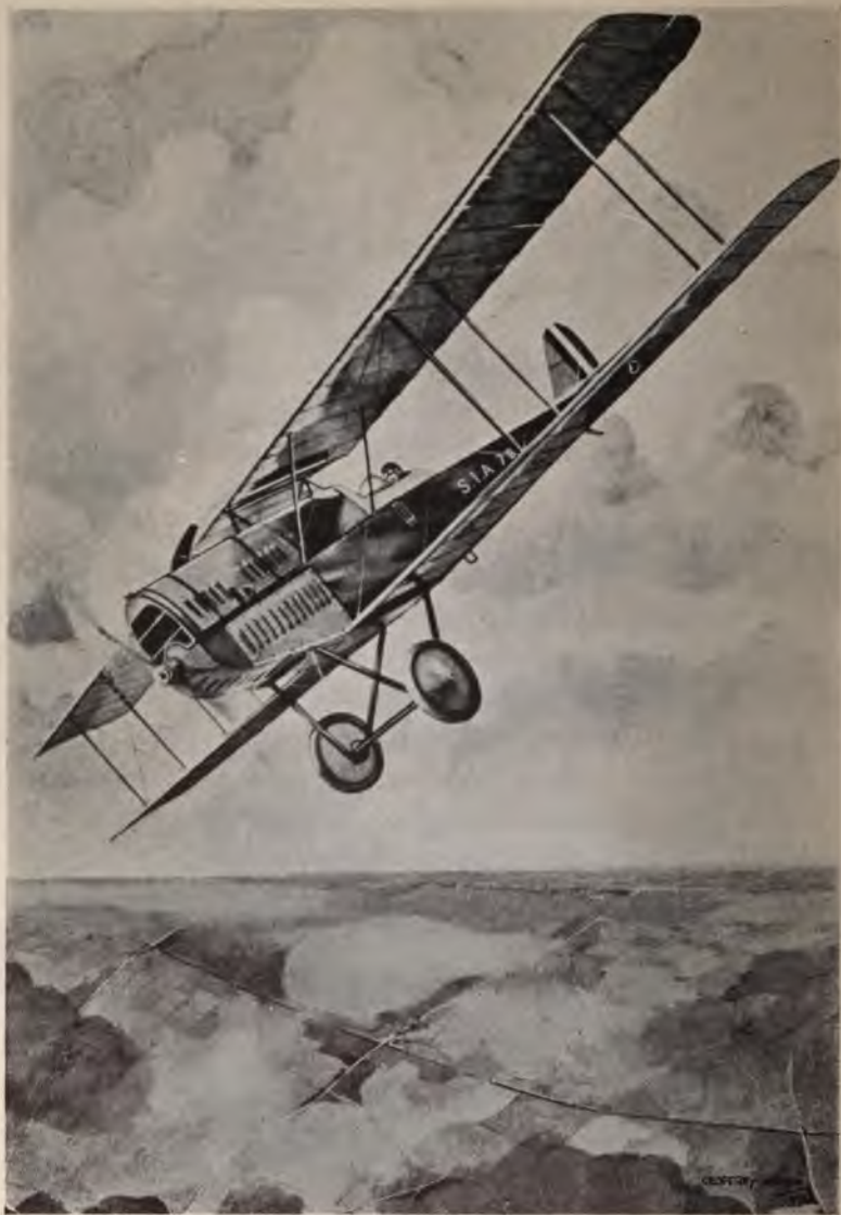
AN ITALIAN AEROPLANE WHICH SECURED MANY RECORDS IN 1917. NOTE THE CAR-TYPE RADIATOR
